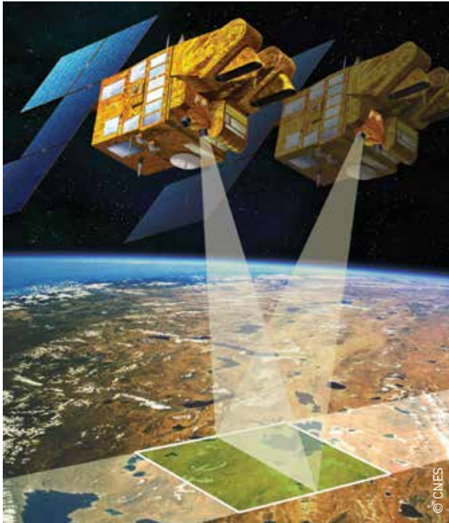
How the HRS instrument works (Spot 5)
